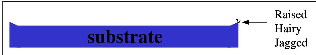
Figure 4 A schematic of the raised edge caused by slitting with blunt blades.
